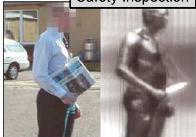
Spot the knife? Millimeter waves, close to terahertz, show their ability to see through clothes and paper.
